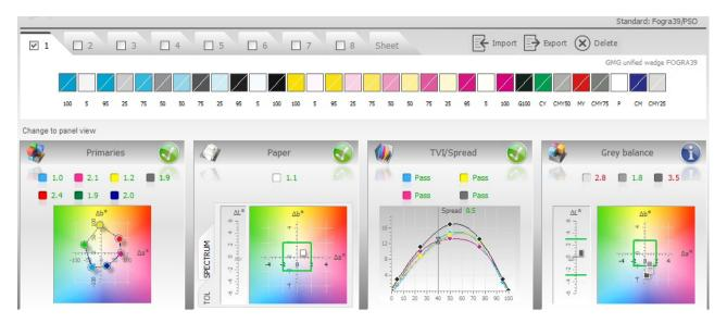
The software tool also recommends the dot gain compensation to be done in prepress RIP to ensure that your press prints within ISO specified dot gains. This also helps in making multiple presses to print with same tones.
